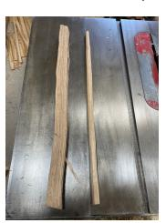
the piece of wood on the right. If it's surgically sharp and you're sufficiently skilled, you can use a drawknife to slice between the grown rings on a piece of wood. That's what you need for spindles (the grain runs the entire length of the spindle).
